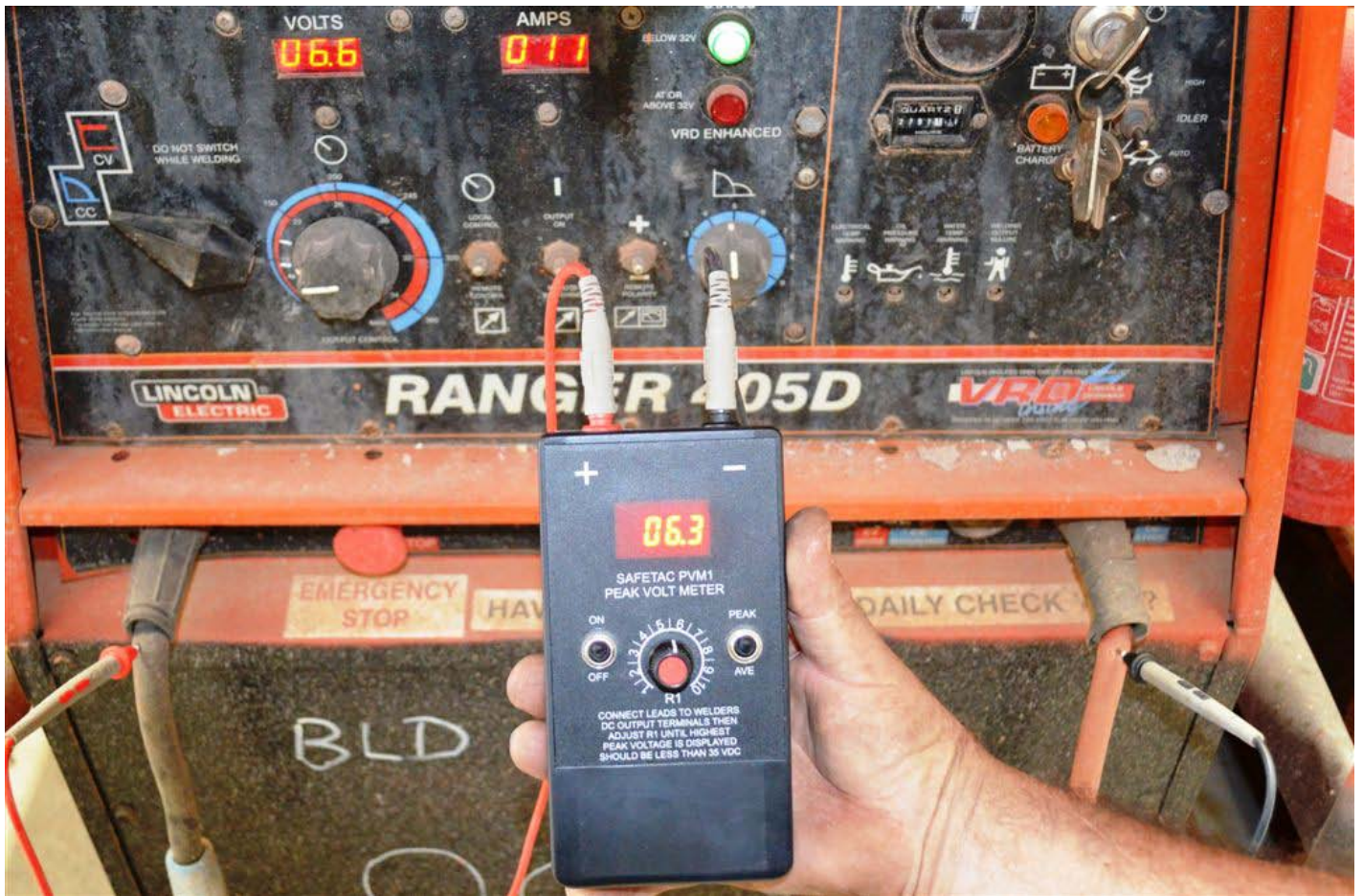
PVM1 testing peak voltage on Lincoln 405D
